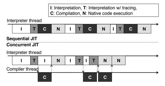
Figure 3.3: Example of sequential vs concurrent JIT execution flow.
