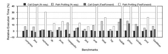
Figure 2.8: Performance of N-way buffering and FastForward relative to CAB. We use N:M threading on an Intel Core 2 Quad. The Y-axis is normalized to CAB's execution time.
