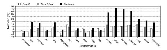
Figure 2.11: Call graph profiling overhead on native threading model with per-processor CAB.
