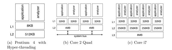
Figure 2.4: Experimental processors data cache structure. Instruction or trace cache is omitted. Application and analyzer's mapping to the cores is idealized, and it is not a requirement.
