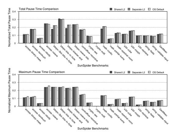
Figure 3.9: Pause time impact on various core configurations.
