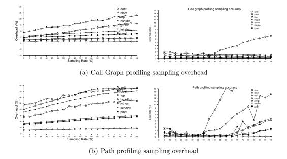
Figure 2.13: Sampling overhead and error rate for call graph and path profiling (N:M threading on an Intel Core 2 Quad).
