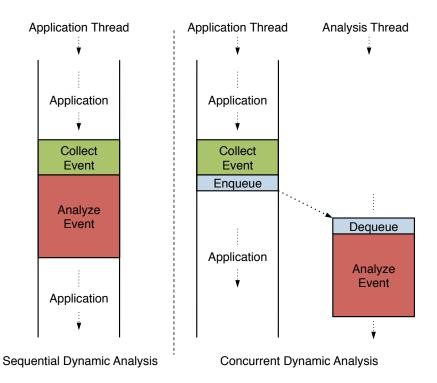
Figure 2.1: Generic sequential dynamic analysis versus concurrent dynamic analysis.
