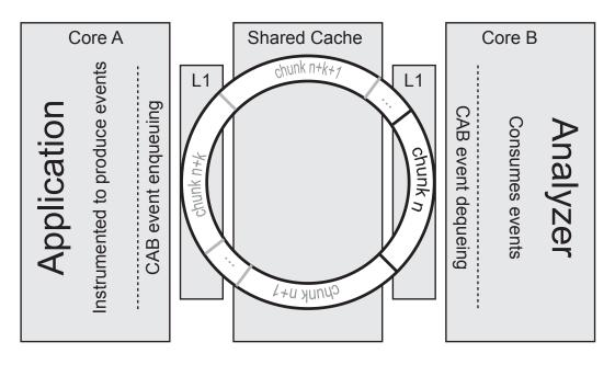
Figure 2.2: Cache-friendly Asymmetric Buffering (CAB) in a concurrent dynamic analysis framework.
