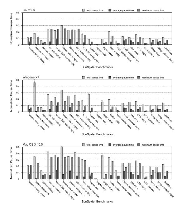
Figure 3.6: Pause time ratios of concurrent vs. sequential JITs.
