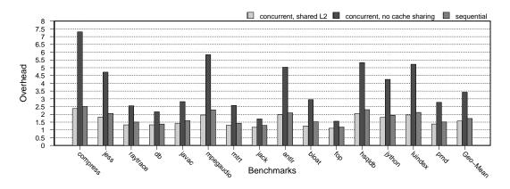
Figure 2.14: The importance of shared caches. Path profiling overhead with and without sharing between analyzer and application threads. Note that y-axis is the factor of overhead, and not a percentage.
