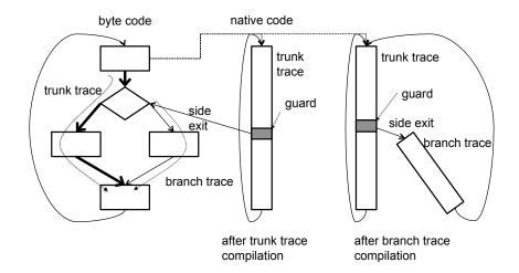
Figure 3.1: Byte code and native code transition in the trace-based JIT. Initially, the interpreter interprets on the byte code. First detected hot path (thick path) is traced forming a trunk trace. Following hot paths guarded and installed in a side-exit. The compiler attach the branch trace, which begins from the hot side-exit to the loop header, to the trunk trace.
