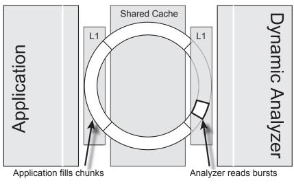
(c) Bursty Sampling. The analyzer samples a burst from each chunk.
