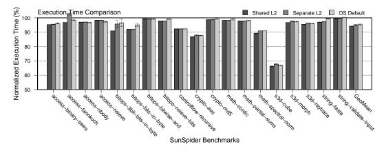
Figure 3.8: Performance impact on various core configurations.
