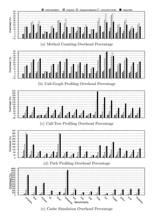
Figure 2.17: Per-benchmark exhaustive mode overhead on Pentium 4 (N:M threading model)
