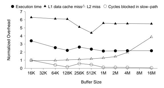
Figure 2.12: Performance as buffer size varies for path profiling on DaCapo hsqldb (using N:M threading on an Intel Core 2 Quad).
