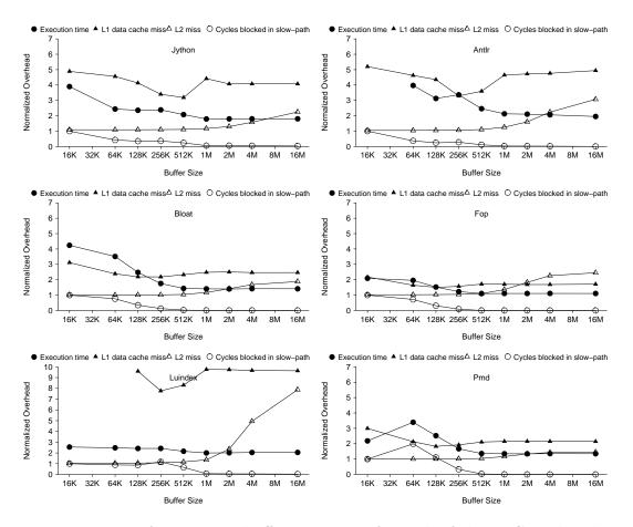
Figure 2.19: Performance as buffer size varies for each of the DaCapo benchmarks. Results are for path profiling using N:M threading on an Intel Core 2 Quad.
