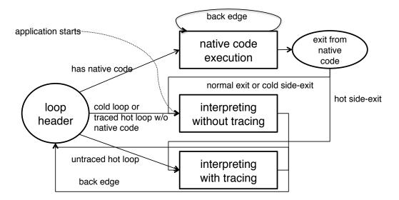
Figure 3.4: The interpreter state transition at a loop header.
