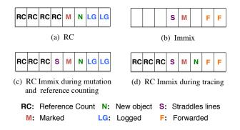
**Figure 2.** How RC, Immix, and the different phases of RC Immix use the eight header bits.
