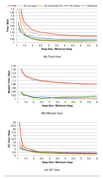
**Figure 4.** The performance of GenImmix, RC, RC Immix, and RC Immix with no proactive copying (No PC) as a function of heap size.
